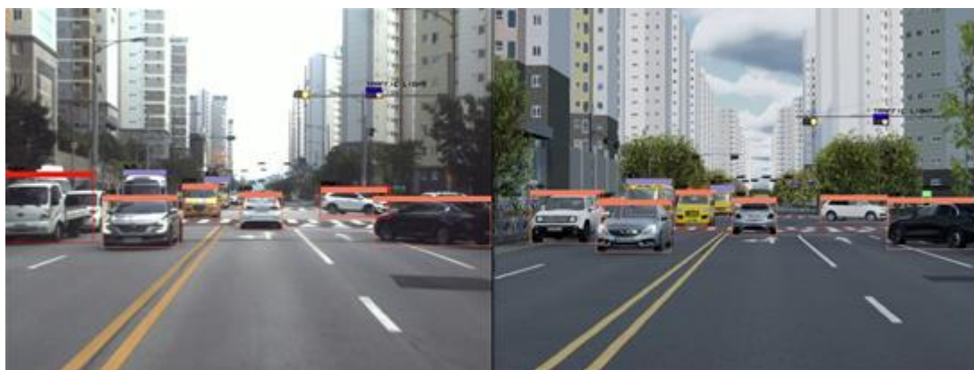
Figure 7: Object detections by YOLOv4 on real-world data (left) compared to simulation data (right) for timeframe 00:03.238
