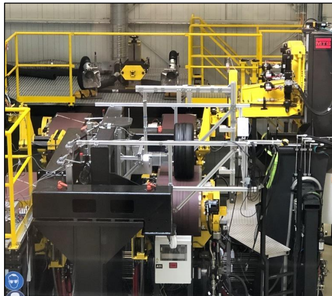
Figure 2: Tyre Deformation Test Bench
