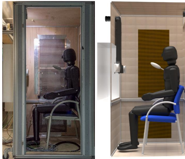
Figure 6: Climate chamber measurement setup (left) and simulation model (right).
