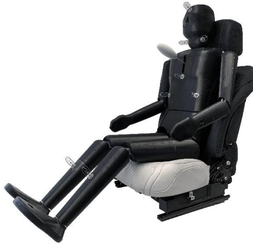
Figure 3: Thermal comfort manikin with sensors on a vehicle seat.
