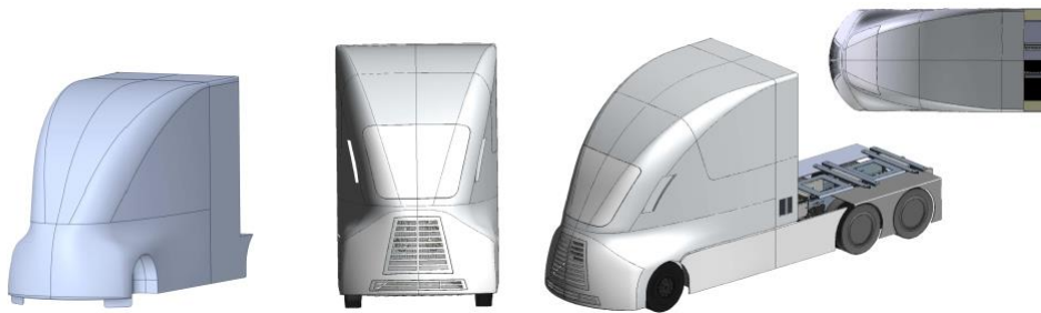
Figure 7: Optimized Aerodynamic model (left), New designed physical 30% scale model (right)
