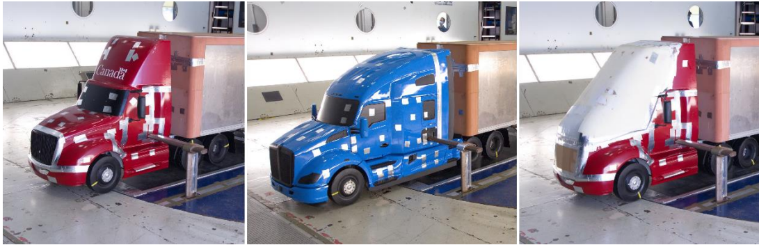
Figure 1: Three wind tunnel tractor-trailer scale models: day-cab tractor(left), sleeper-cab tractor (middle), and zero-emission-cab tractor (right)
