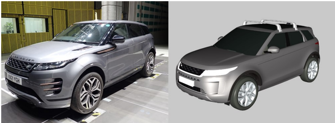
Figure 3: The vehicle under test in the wind tunnel and virtual representation
