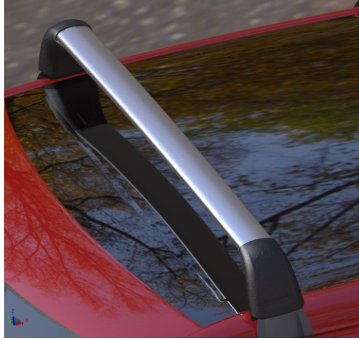
Figure 10: A rendering of the roof bars with the T-track cover removed and the cavity tangentially covered
