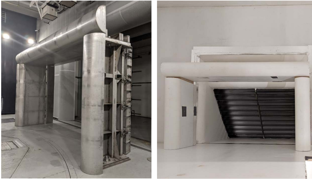
Figure 3: The new stand-alone collector (left) and a model scale version, rotated 90 degrees (right)
