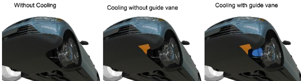
Figure 7: Illustration of brake cooling design on AeroSUV
