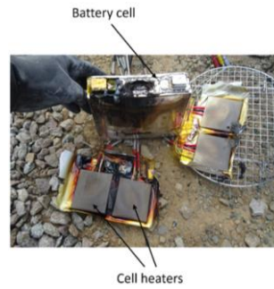
Figure 7: Battery cell and heaters after Thermal Runaway (TR) event.
