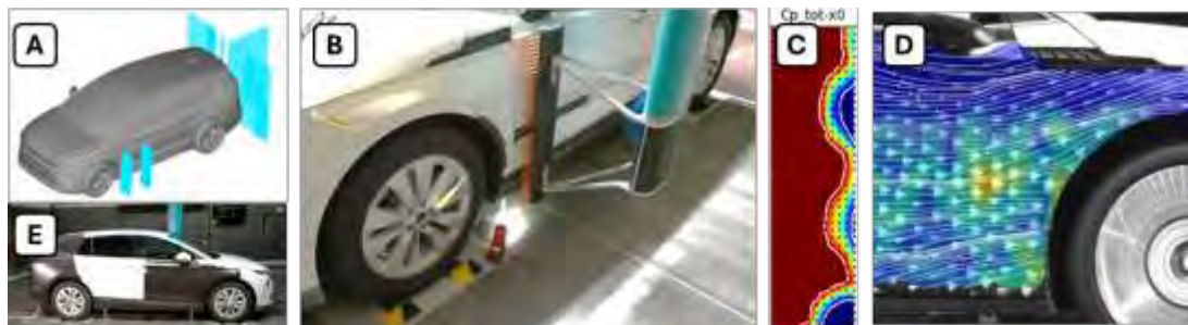
Figure 2: Př Overview of optimized areas within the facelift (A – wake traversing zone, B – traversing arm monitoring the wake behind the front wheel, C – visualization of the measured total pressure field behind the front wheel, D – visualization of measured flow fluctuations using video analysis of yarn oscillation, E – overall view of the experimental vehicle in the aerodynamic tunnel)
