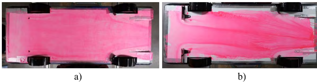
Figure 8: Wall shear patterns for the configurations a) without_WS and b) with_WS . Flow goes from left to right.
