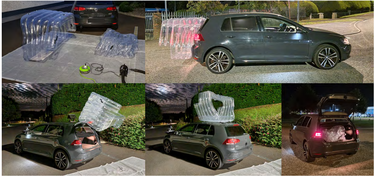
Figure 8: Images highlighting the adapted (inner-removed) inflatable double cavity device for the VW Golf. Shown is an outline for how the inner cavity was cut away and how the device can be manoeuvred to facilitate access to the rear boot space and how it can be easily deflated and stored.
