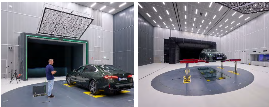
Figure 2: Test section showing vehicle operating with wheel spinners, and frontal array above the nozzle (left) and view looking downstream with the glass floor installed and the control room window visible (right)
