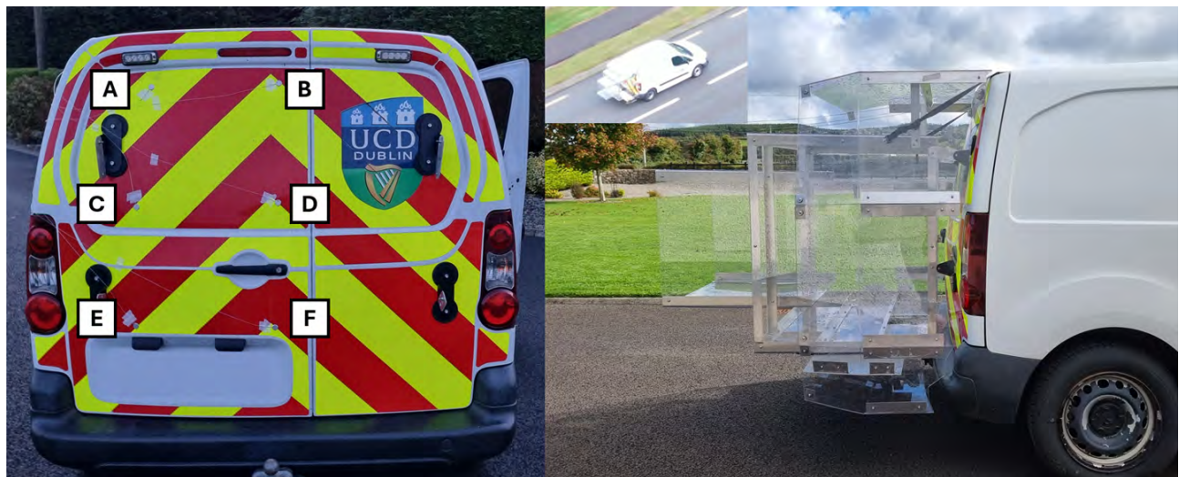
Figure 9: Images showing the locations of the six base pressure patches fitted to the Citroen Berlingo van (left) and the rigid triple cavity device fitted to the van for testing (right).
