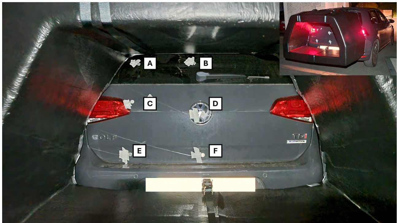
Figure 10: Locations of the six base pressure patches fitted to the VW Golf Mk7 during the surface pressure testing with the foam cavity device.
