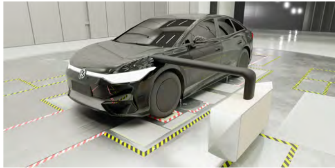
Figure 2: Concept of the measurement setup enabling PSP testing on the road.
