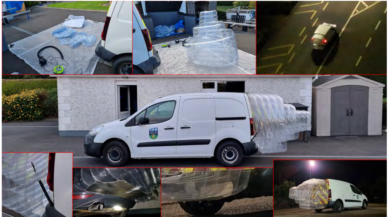
Figure 3: A collection of images highlighting the inflatable triple cavity device for the van. This figure demonstrates the inflation process, how it is protected from hot exhaust gases (with an image of the shield on the VW Golf Mk7 for a better visual), and how it looks on the road from an aerial view.
