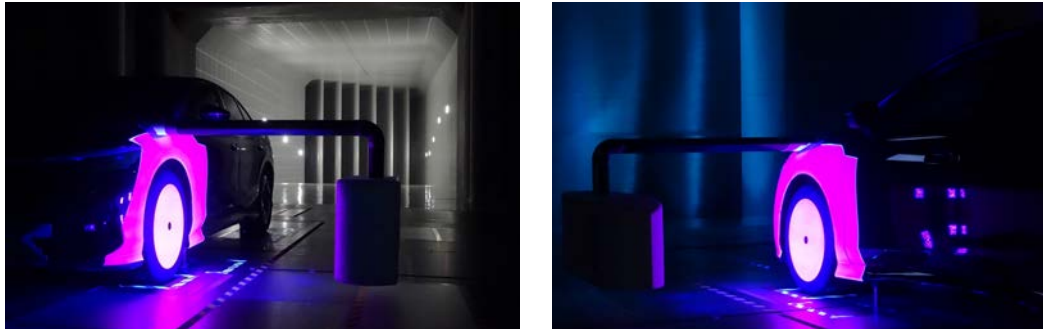
Figure 6: Setup in the AAK with activated UV LED spotlights.
