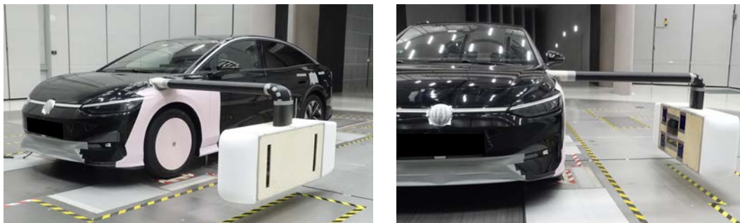
Figure 5: ID.7 in the AAK including measurement equipment.
