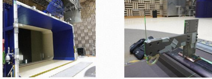
Figure 13. VG and pitot tube set-up in HAWT
