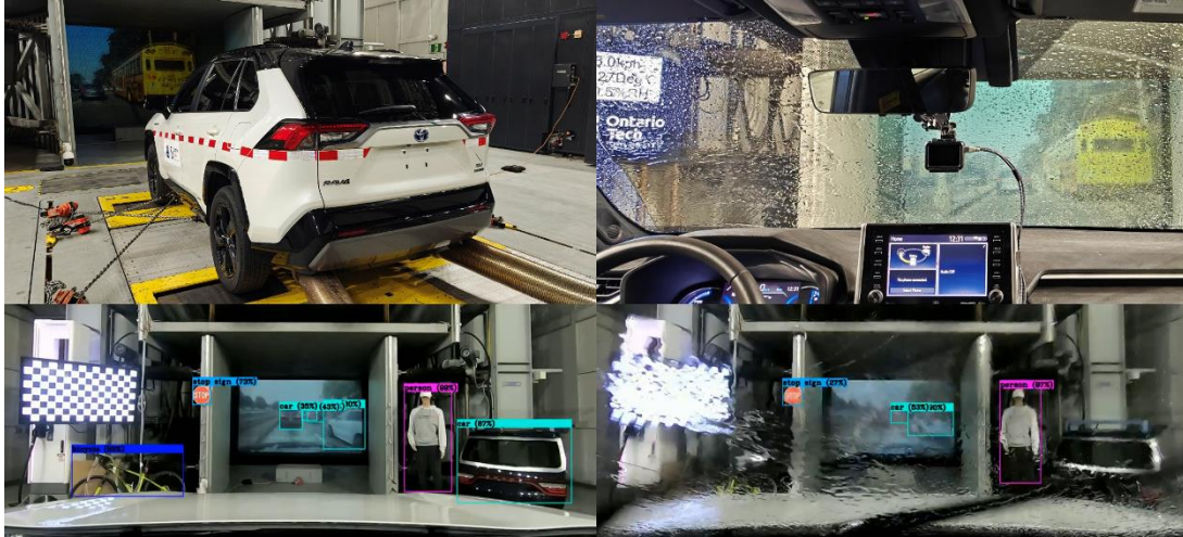
Figure 6: Dynamic display with physical rain simulation hybrid digital twin platform. Sample object detection quality on dynamic and static targets.
