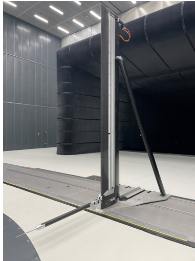
Figure 11: Flow Uniformity Measurement Rig at the X = 4.5 m Test Plane
