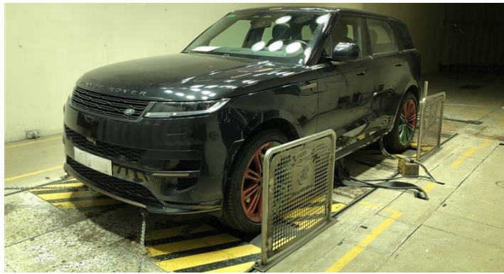
Figure 1 – Image of a chassis dynamometer within a CWT
