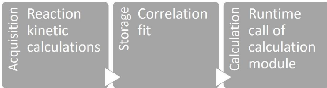
Figure 1: Schematic structure of the automated approach to handle ignition delay times from different fuels in simulation. [8]
